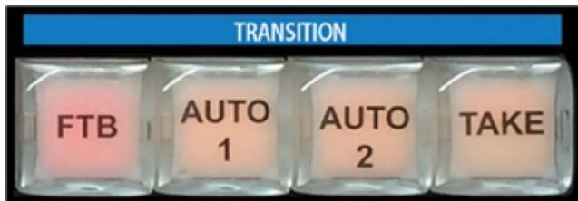
In live switching, changing from one camera or clip to another is called a transition. The vMix Control Surface has three available transition types available, corresponding to transition buttons in vMix.
