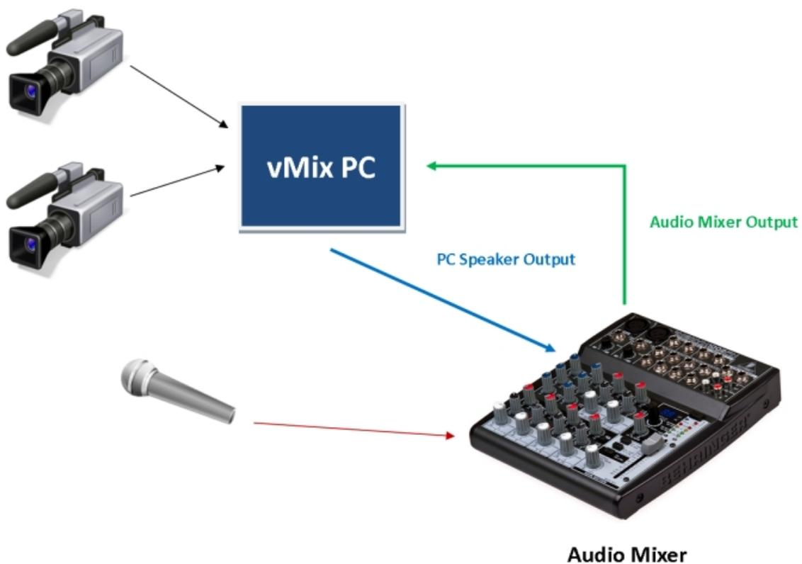
In the diagram above, all external audio sources such as Microphones are connected to a separate external **Audio Mixer**.
