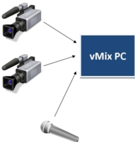
In the diagram above, all audio sources such as Microphones and Cameras run directly into vMix.
